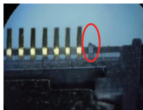
Molding件端子缺Pin PinMolding Parts Lack Pin
