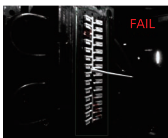
一次检测出定模粘模(产品缺料) First detects cores sticking (absence parts)
