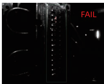
二次检测模具动模粘模 Second detects sliders sticking
